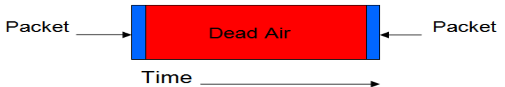
Figure 17: Actual Overhead of IEEE 802.11n Carrier Sensing for Single Packets Sent at High Rate 59
