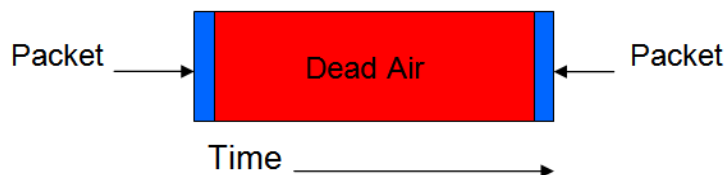
Figure 11 Actual overhead of IEEE 802.11n carrier sensing for single packets sent at high rate. 18
