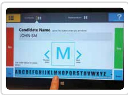
*The EZ Ballot, a winning concept in the OpenIDEO challenge was developed in a graduate-level design class at the Georgia Institute of Technology. The final design combines tactile buttons, audio prompts, touch screen interaction and a slider for text entry.*
