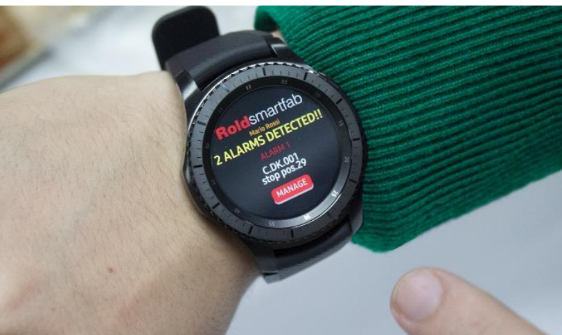
Real-Time Notification to the Operator
