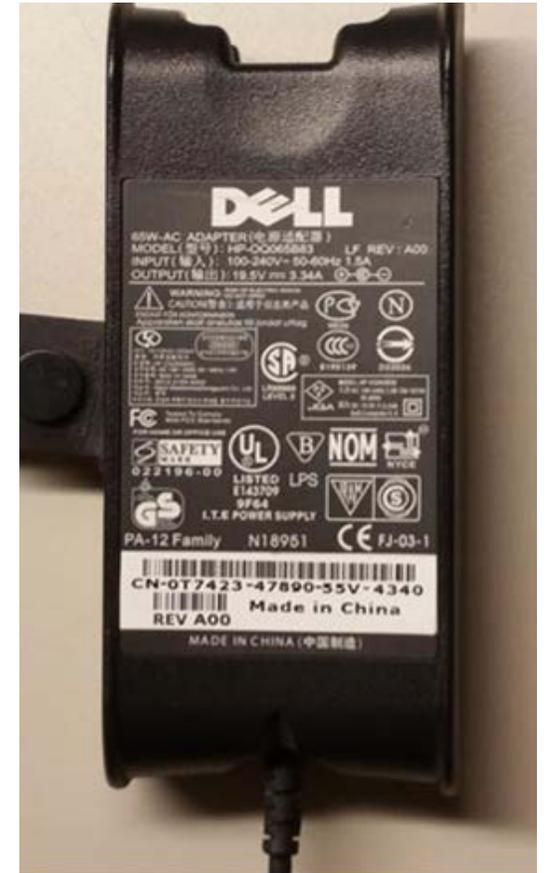
Figure 1. Compliance labeling on a computer power supply may be provided in different ways.
